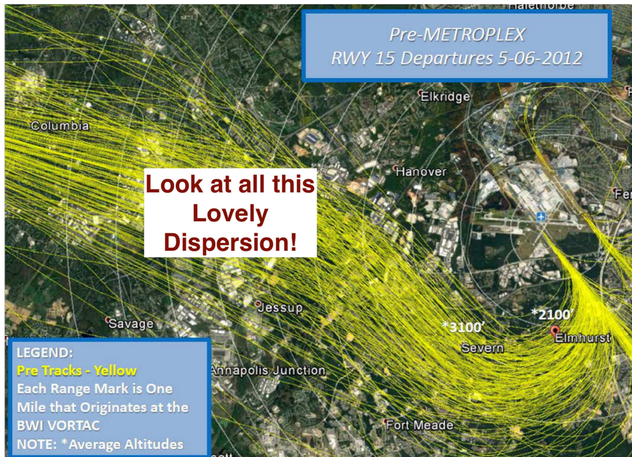
Figure 2B Runway 15 Departures – shows pre-DC Metroplex/NextGen features that need to be restored.
