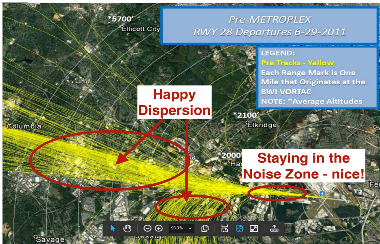
Figure 1B Runway 28 Departures – shows pre-DC Metroplex/NextGen features that need to be restored.
